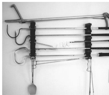
Keeping your tools handy near the room entrance is a wise idea. (pic- A.Hunter) Shown from top to bottom: 40" grab stick (Pilstrom tongs), 44" & 40" hooks, 16" juvi hooks, 40" feces spoon, 36" hook, 18" locking forceps, 14" feces spoon and wire hooks for neonates. Also shown is the wall mountings, which are really fishing pole holders screwed to the wall, and I found perfect for the purpose. All tools should be hung on the wall out of the way, so as to avoid floor clutter for handling. Another good idea is to have your tools located just inside the room entrance for fast access, should a snake be loose in the room (let's hope not!). (pic- E.Wainberg)
