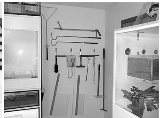
Keeping your tools handy near the room entrance is a wise idea. (pic- A.Hunter) Shown from top to bottom: 40" grab stick (Pilstrom tongs), 44" & 40" hooks, 16" juvi hooks, 40" feces spoon, 36" hook, 18" locking forceps, 14" feces spoon and wire hooks for neonates. Also shown is the wall mountings, which are really fishing pole holders screwed to the wall, and I found perfect for the purpose. All tools should be hung on the wall out of the way, so as to avoid floor clutter for handling. Another good idea is to have your tools located just inside the room entrance for fast access, should a snake be loose in the room (let's hope not!). (pic- E.Wainberg)
